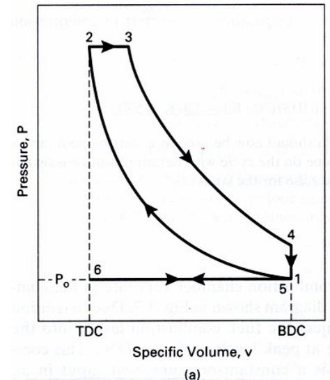
Process 4-5—constant-volume heat rejection (exhaust blowdown).
