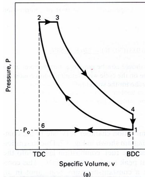
$$\beta = V_3/V_2 = v_3/v_2 = T_3/T_2$$
