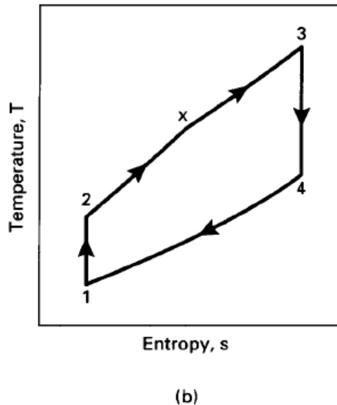
**Figure 3-10** Air-standard Dual cycle, 6-1-2-x-3-4-5-6, which approximates the four-stroke cycle of a modern CI engine on (a) pressure-specific volume coordinates, and (b) temperature-entropy coordinates.
